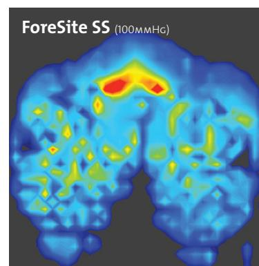
ForeSite SS shows exactly where the pressures are that require relief. With 1296 pressure sensing points on an 18" x 18" (45cm x 45cm) sensor, no other sensor comes close to the resolution of the LX100.
